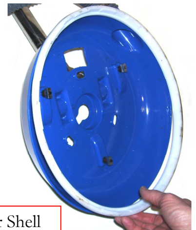
Remove the Brush Ring or Hard Boot
