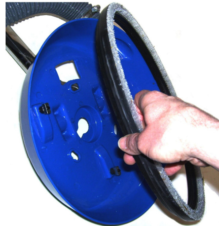
Remove the Brush Ring or Hard Boot
